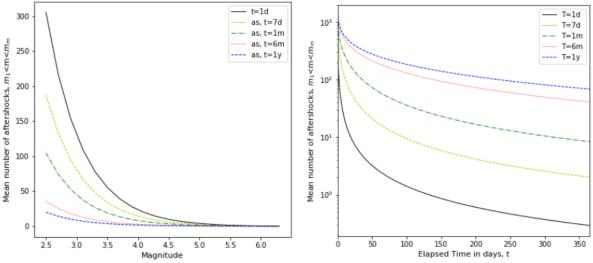
Fig. 5 - Mean number of aftershocks with magnitude m, for different time frames.
