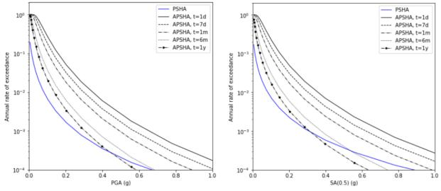
Fig. 9 - Comparison of mainshock and aftershock site hazard curves at Elbasan city for a different elapsed interval from the occurrence of the main event. Left: PGA. Right: SA(0.5).
