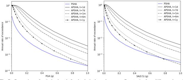
Fig. 7 - Comparison of mainshock and aftershock site hazard curves at Durrës city for a different elapsed interval from the occurrence of the main event. Left: PGA. Right: SA(0.5).
