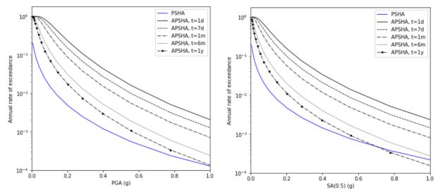
Fig. 8 - Comparison of mainshock and aftershock site hazard curves at Tirana city for a different elapsed interval from the occurrence of the main event. Left: PGA. Right: SA(0.5).
